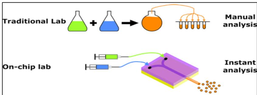
Fig. 3. Comparison between traditional and microfluidic diagnostics. Redrawn from: Brivio, M., Verboom, W., 7 Reinhoudt, D. N. (2006). Miniaturized continuous flow reaction vessels: influence on chemical reactions. *Lab on a chip*, 6, p.239.
